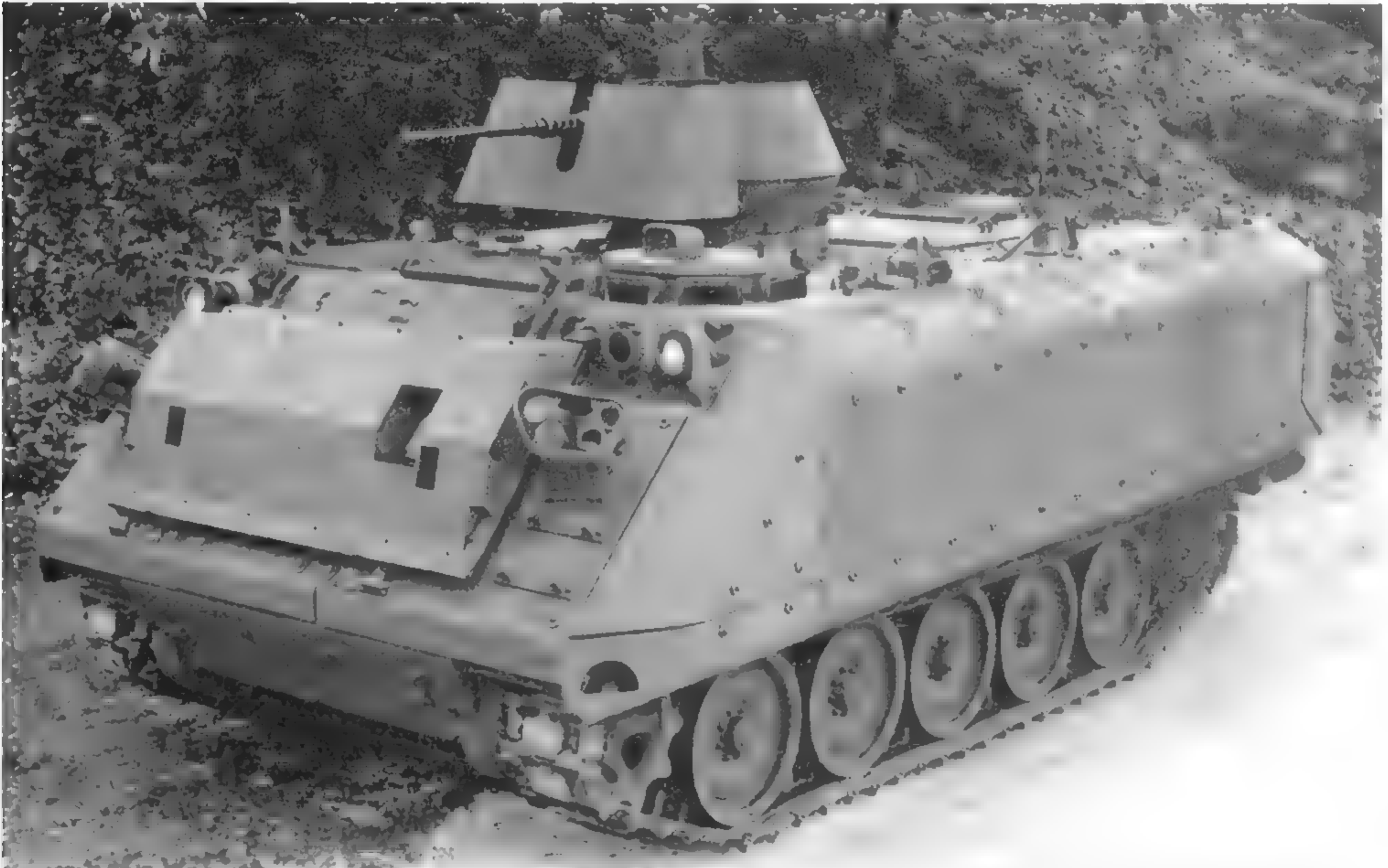
The M113A3 was fitted with the P-900 applique armor kit, resulting in the first truly noticeable change to the vehicle's form since its inception. (U.S. Army photo)
